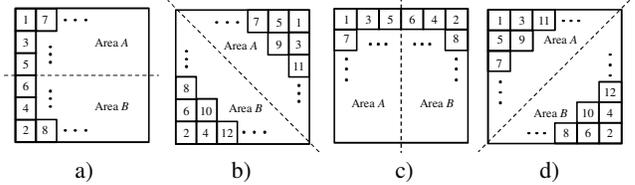
Fig. 3. Partitioning of a sub-band into areas  $A$  and  $B$  and processing order of blocks according to the global symmetry: a) horizontal, b) diagonal-down, c) vertical, and d) diagonal-up
