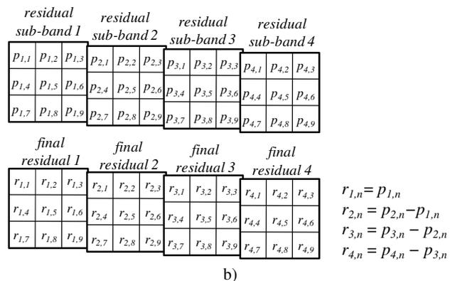
Fig. 5. a) The five proposed prediction modes for inter-slice DPCM prediction: 1. Horizontal, 2. Down-45°, 3. Up-45°, 4. Left-45° and 5. Right-45°. b) Calculation of the final residual data for a group of  $3 \times 3 \times 4$  samples using the horizontal prediction mode.  $p_{s,n}$  denotes the  $n$ th sample of residual sub-band  $s$ ; and  $r_{s,n}$  denotes the  $n$ th final residual sample of sub-band  $s$ .
