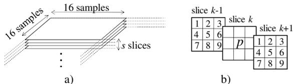
Fig. 4. a) Group of  $16 \times 16 \times s$  samples used in inter-slice DPCM prediction. b) Sample  $p$  in slice  $k$  and its nine immediate neighbors in slice  $k-1$  and slice  $k+1$ .
