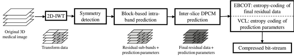
Fig. 1. Block diagram of the proposed scalable lossless compression technique. 2D-IWT: two-dimensional integer wavelet transform. DPCM: differential pulse code modulation. EBCOT: embedded block coder with optimized truncation. VCL: variable length coding.
