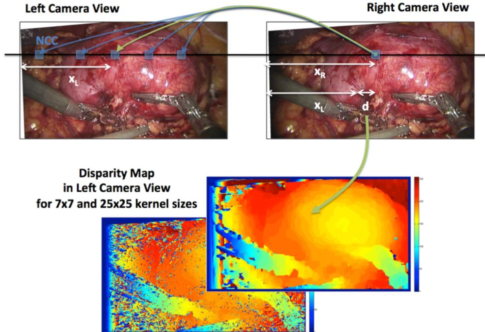
Fig.1(a) - Correlation-based dense matching between left and right camera view. Normalized Cross Correlation (NCC) ratio is computed between left and right images along an epipolar line (in black). The disparity is the distance between the two matching points along this epipolar line.
