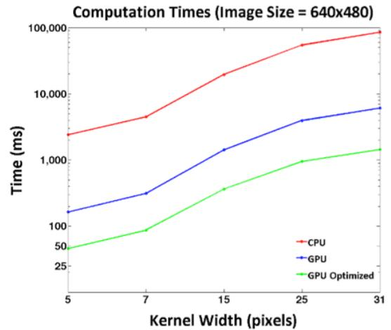
Fig.1(c) - Computation times (in ms) of CPU, GPU and GPU optimized implementations for an image size of 640x480 with respect to kernel sizes.
